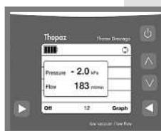
3. Change into standby mode: press “Off” button for a min. 3 sec.
